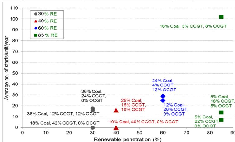
The impacts of the operational constraints modelled depend particularly on the level of carbon price and the mix of generation technologies within the portfolio.
