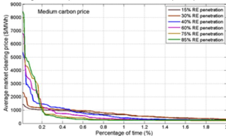
The reduction in spot prices results in reduced revenue and profit of generators and potentially leads to insufficient revenue. The revenue impacts on large-scale PV are very severe at high renewable penetrations. Changes in market mechanisms (such as a higher market price cap) are likely to be required to ensure long-term resource adequacy and revenue sufficiency in an energy only market.
